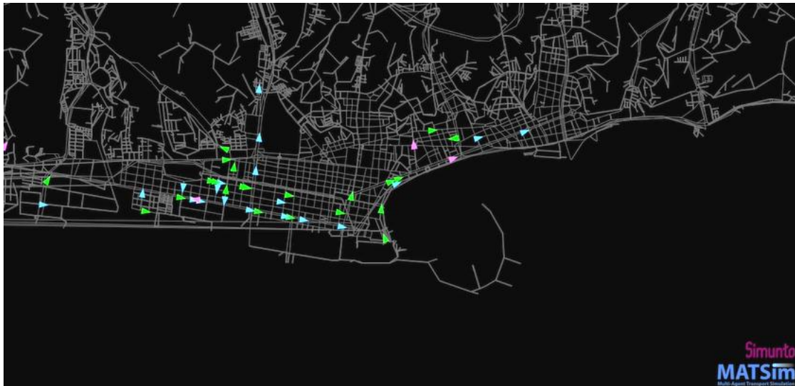
Figure 24 - A detail of the Messina road network, showing the central part of the city. Simulated vehicles are included, where pink triangles represent public transport, green ones cars and blue ones cyclists.
